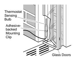
Figure 51 - Installing Thermostat Sensing Bulb behind Glass Doors
